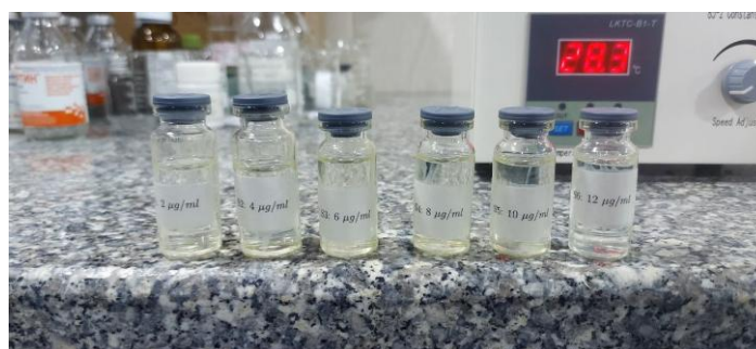
Figure 2: Standard solutions of diclofenac sodium in phosphate buffer solution
